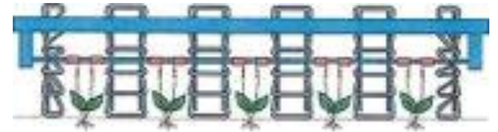
Fig.3 - Scheme of the association of the active disc harrow with elastic herbicides, to carry out selective weed control interventions both in the inter-row and on the row.
