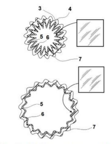
1 = artificial bladder; 3 = internal layer (non-polymeric), with high resistance to urine; 4 polymeric layer; 5,6 = foldable recesses and crests, 7 = biocompatible coating
