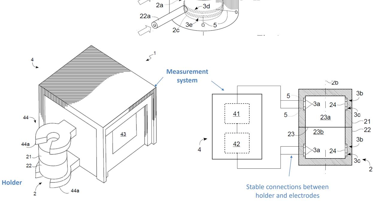
Integral electrodes with the chamber 21\_
