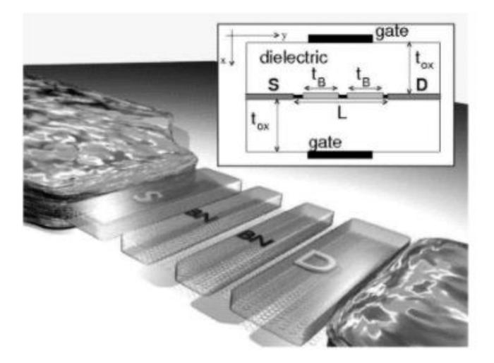
Second realization of a resonant tunnel FET (RTFET), where two hBCN domains of length tB are present in the channel and below the gate, separated by a graphene region of length w.
