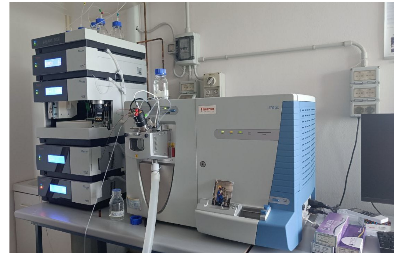
HPLC Dionex UltiMate 3000 with auto-sampler coupled with a Thermo Scientific LTQ XL MS
