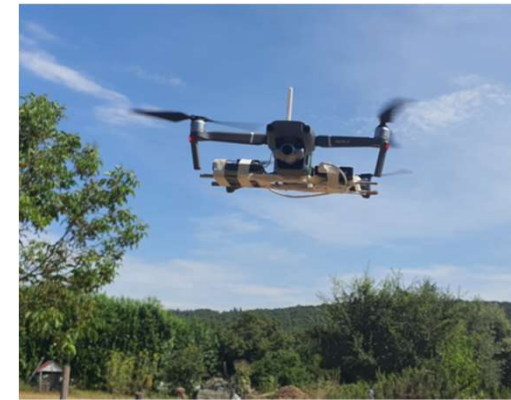
UAV DJI Mavic 2 with LoRa gateway onboard
